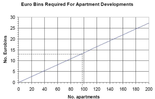
**Figure 2:** Bulk Waste Container Sizes (Euro Bins)
